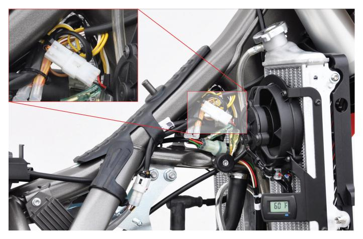
7.) Connect fan kit to bike power. If the motorcycle came from KTM with the fan harness then the Trail Tech fan kit will plug directly into the factory connector. This is located just to the left of the radiator in the wiring above the motor (See above photo). If the motorcycle did not come with a factory harness, then install the provided power lead for the fan kit. Connect the ring terminals directly to the machine's battery (Black to negative, red to positive).
